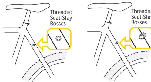
This rear carrier is designed to fit bicycles with threaded seat-stay bosses. The mounting bracket arms are designed to fit a wide range of bicycles sized from 26" wheel x 14.5" frame to 700C wheel x 63 cm frame.
