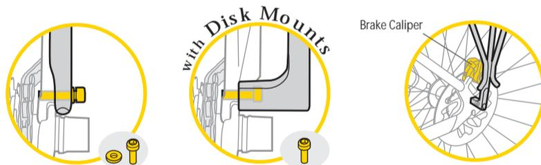
1. When installing Rear Rack, check that the bolts will not interfere with the brake caliper, chain, or cog set before completely tightening them. Tighten all bolts to 6-8 Nm (53-69 in-lbs) before loading Rear Rack.
