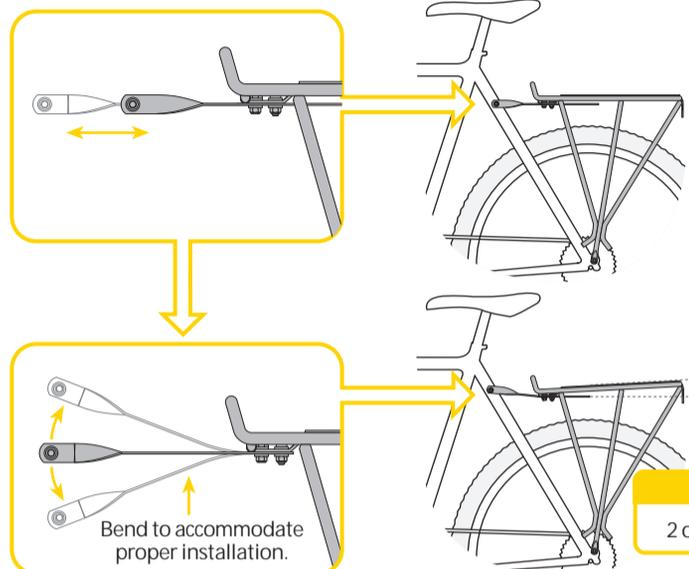
1. Attach the mounting bracket arms to the front of your One Fits All REAR RACK as shown. Don't tighten completely at this time.
