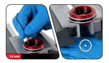
Remove and replace the bottom out washer and o-ring from the shaft.
