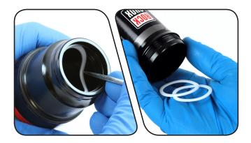
Spray isopropyl alcohol inside the air can and clean it with a rag. Remove a glove and use your finger to inspect the inside and outside of the air can for scratches, dents, or other surface deformations. Replace the air can if it is scratched or damaged.
