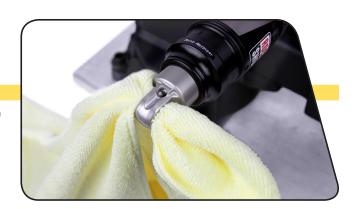
Use a strap wrench to remove the air can. Wrap the strap around the section of the air can furthest from the shaft eyelet. Turn the wrench counter-clockwise to unthread the air can.
