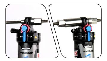
Clamp the catcher in a vise or hold it secure with a 13 mm wrench.
