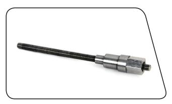
Insert the threaded rod through the bushing pin then through the shaft eyelet so that the bushing pin is positioned between the push pin and the eyelet.
