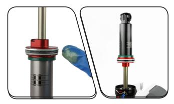
Apply a small amount of grease to the air can threads. Inject 0.5 mL of Maxima® Maxum4 Extra 15w 50 into the air can before installing the air can onto the damper. Firmly press the air can down until the sealhead/air piston is inserted into the air can.
