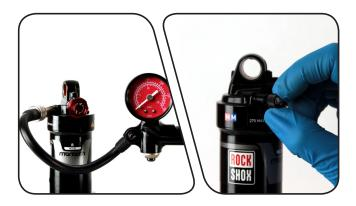
DebonAir™ Air Cans only: Use a shock pump to pressurize the shock to the desired air pressure. After adding air to the shock, the pressure will need to be equalized between the shock chambers.
