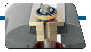
Monarch™ RT3: Use a 12 mm socket wrench to remove the piston nut.
