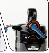
Use a Schrader valve tool to remove the damper air/nitrogen fill port cap. Use a small hex wrench or pick to depress the Schrader valve and release all air pressure from the damper.
