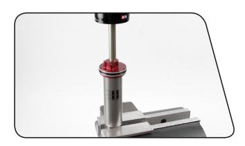
Use a 2 mm hex wrench to remove the bleed screw, located in the seal head/air piston.
