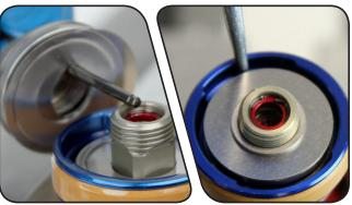
Monarch R: Install the main piston assembly that was removed in step 5 onto the damper shaft.
