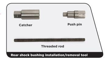
Thread the small end of the push pin onto the threaded rod until the rod is flush or slightly protrudes from the hex-shaped end of the push pin.
