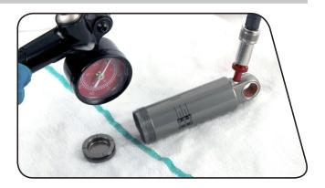
2 Spray isopropyl alcohol on the inside and outside of the damper body and clean it with a rag.
