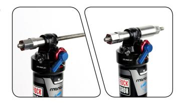
Clamp the catcher in a vise or hold it secure with a 13 mm open end or adjustable wrench.
