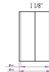
For 50mm OD head tube. 1 1/8" Internal Standard
