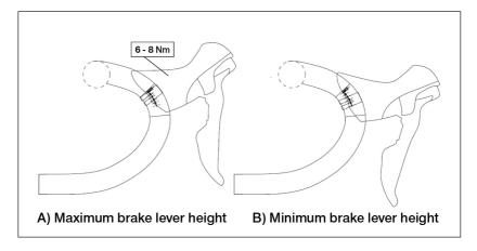
**WARNING:** Never rotate levers on a handlebar after you have significantly tightened the clamp bolts, or you will scratch its surface marring the finish and potentially risk damaging the handlebar.
