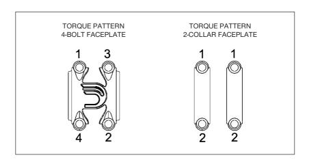
Check the symmetry and equality of all the distances between faceplate, body, handlebar stem, if necessary, further tighten up to 5 N • m.
