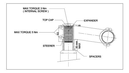
The drawing above shows the correct fitting of the handlebar stem on the fork steerer. Cutting the fork steerer to size is a delicate operation and can release harmful particles, irreparably damaging the fork itself if done without the proper equipment.
