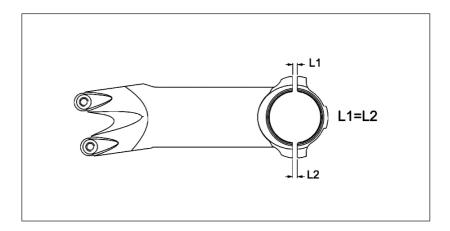
Then, using a torque wrench, tighten the bolts alternately in a cross pattern, turning ½ turn at a time.
