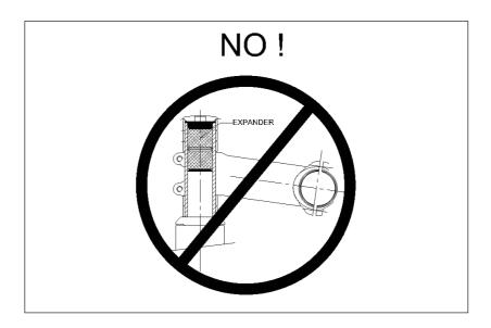
Install the expander in the fork steerer until it stops, and tighten the expansion bolt at maximum torque of  $3 \text{ N} \cdot \text{m}$ .
