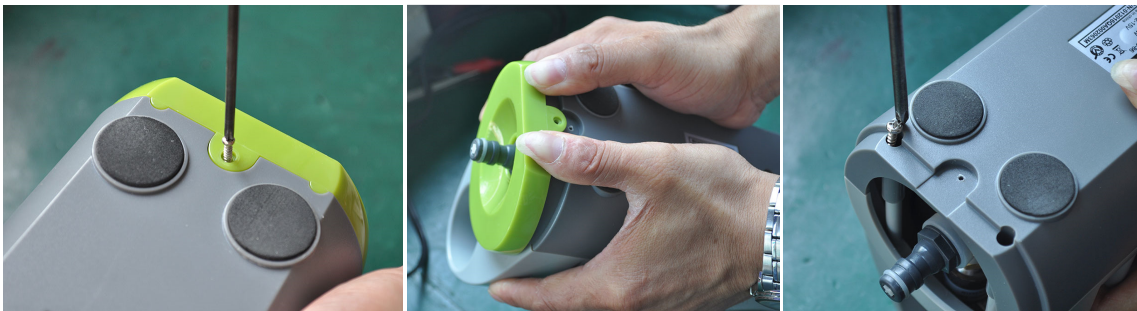
Unscrew these 5 pcs of screws highlighted on above photo on the bottom to open the housing
