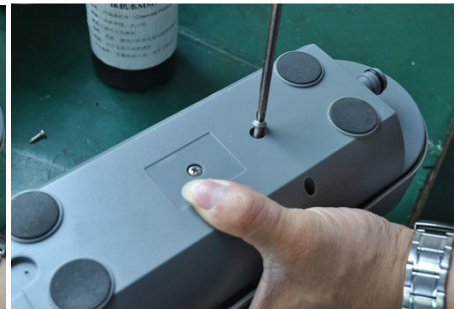
Tear off the rating label, and screw off to release the pump
