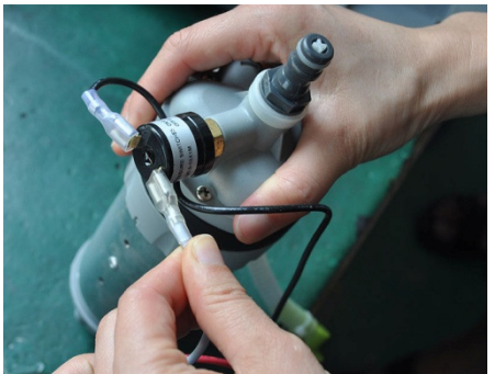
Disconnect the wire on pressure switch
