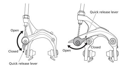
For models with a CLOSE position mark on the quick release lever and brake body side, adjust the position of each mark so that they are aligned. At this time, check that you can feel a click.
