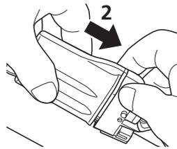
Install the battery so that it follows the groove in the battery mount.
