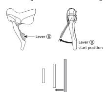
Push the lever up to the stopper and then release it.
