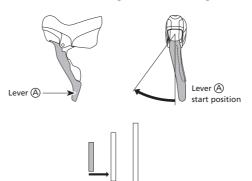
Push the lever up to the stopper and then release it.
