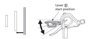
"You can shift gears either by pushing or pulling the lever."
