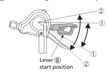
"You can shift gears either by pushing or pulling the lever." Some models allow two-step gear shifting.
