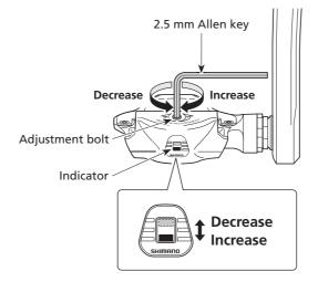
Do not turn the bolt past the point at which the indicator shows the maximum or minimum tension.
