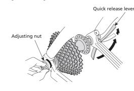
3. Grip the rear end with your fingers and use the palm of your hand to close the quick release lever with as much strength as possible. When closed, the quick release lever must be in the "CLOSE" position shown below in the diagram on the right. The side of the lever with the inscription "CLOSE" must be facing away from the bicycle, and the lever should be parallel to the rear end as shown below in the diagram on the left.
