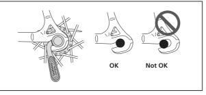
2. Open and close the quick release lever with your right hand while gradually tightening the adjusting nut with your left hand in the clockwise direction. Continue tightening the nut until you feel resistance with your hand at the point when the lever is parallel to the hub (as indicated by the dotted position in the diagram on the right).
