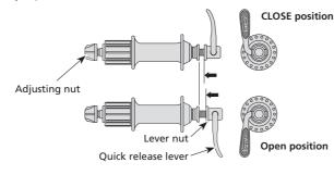
The clamping strength is adjusted by turning the adjusting nut. When the nut is turned in a clockwise direction, the clamping strength increases, and when the nut is turned in a counter-clockwise direction, the clamping strength decreases.
