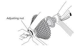
• If the clamping strength is adjusted too strong and the quick release lever cannot be pushed to the CLOSE position, turn the adjusting nut in a counter-clockwise direction to reduce the clamping strength. When doing this, do not fully release the adjuster nut. Turn it 1/8 of a revolution, and then try to push the lever to CLOSE, to set the maximum clamping strength with which you can push the quick release lever to the CLOSE position.
