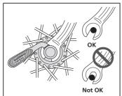
2. Open and close the guick release lever with your right hand while gradually tightening the adjusting nut with your left hand in the clockwise direction. Continue tightening the nut until you feel resistance with your hand at the point when the lever is parallel to the hub (as indicated by the dotted position in the diagram on the
