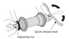
3. Grip the fork with your fingers and use the palm of your hand to close the quick release lever with as much strength as possible. When closed, the quick release lever must be in the "CLOSE" position shown below in the diagram on the right. The side of the lever with the inscription "CLOSE" must be facing away from the bicycle, and the lever should be parallel to the fork as shown below in the diagram on the left.
