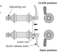
The clamping strength is adjusted by turning the adjusting nut. When the nut is turned in a clockwise direction, the clamping strength increases, and when the nut is turned in a counter-clockwise direction, the clamping strength decreases.
