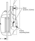
Secure the two bolts with a length of wire as shown in the illustration in order to prevent the bolts from
