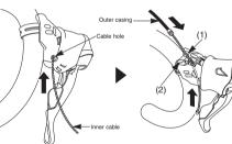
When removing parts in order to replace the inner cable, the work can be carried out more easily if the unit cover is removed as shown in the illustration
