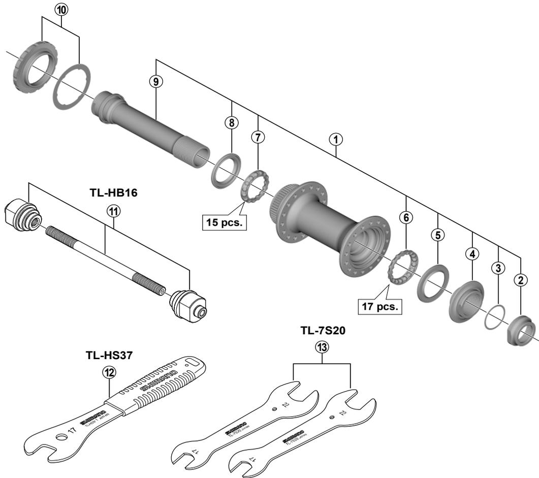
• Over Lock Nut Dimension: 100 mm (3-15/16") for HB-M618 / 110 mm (4-11/32") for HB-M618-B
