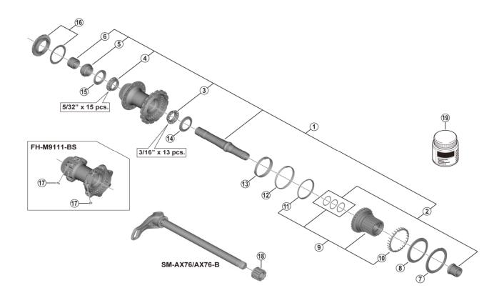
• Over Lock Nut Dimension: 142 mm (5-19/32") for FH-M9111 / 148 mm (5-13/16") for FH-M9111-B, and FH-M9111-BS
