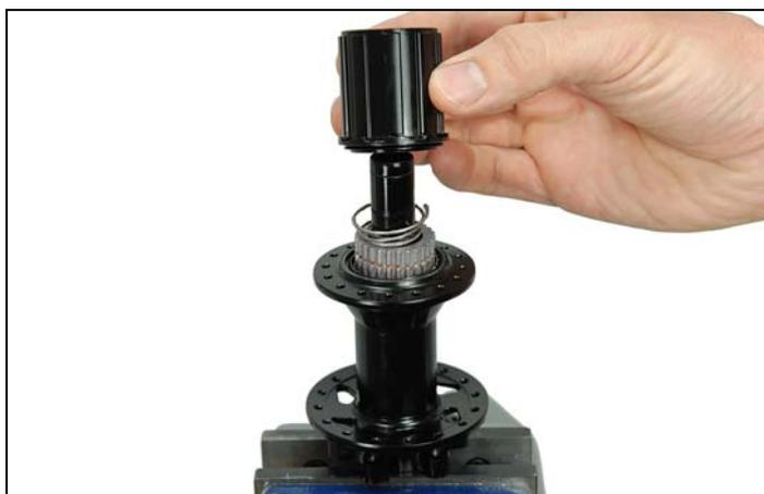
3. Grease both bearings and the contact surface of the end caps (fig. 4-1/1/13).
