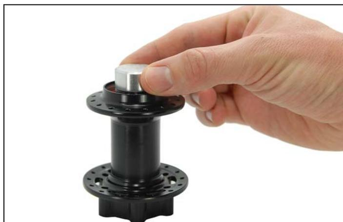
2. Tap the bearing (fig. 3-1/2) and the axle out of the hub shell using the disassembly tool and a hammer.
