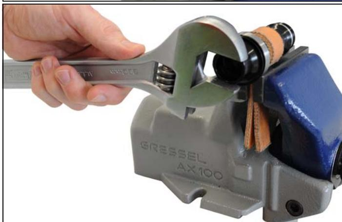
5. Remove the bearing from the axle.
