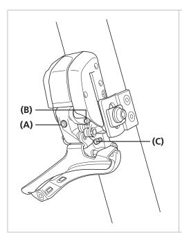
The low adjustment bolt, the top adjustment bolt and the support bolt are close to each other.
