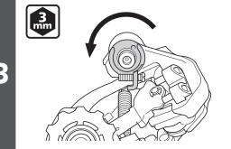
Hold the stopper plate with pliers and turn it counterclockwise.
