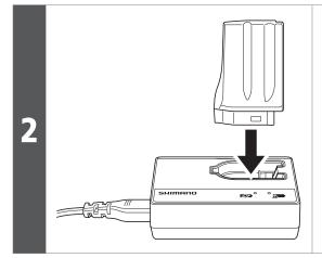
Insert the battery (SM-BTR1) into the battery charger (SM-BCR1) as far as it will go.
