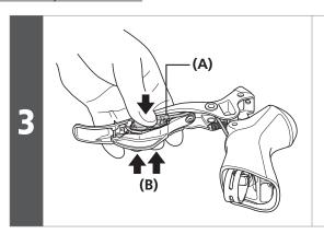
Press the switch unit by hand so that the switch springs go into the grooves in the buttons, and then push the shifting switches [X] and [Y] in as far as they will go.
