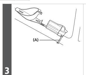
Tighten the bolt of the bottle cage to secure the battery mount.
