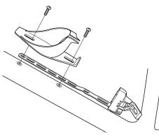
For the long type, secure it with the bolts supplied with the frame or the bottle cage.
