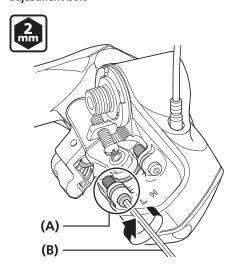
Shift the rear derailleur to the largest sprocket, and then tighten the low-side stopper adjustment bolt until it just touches the left link.
