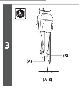
Use a 5mm hexagon wrench to secure the chain guide outer plate so that the flat part of the plate is directly above the largest chainring and so that the rear edge of the chain guide is within 0.5 - 1mm from the front edge.
