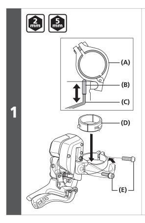
Install the clamp band to the front derailleur.
