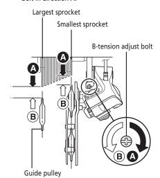
Change to adjustment mode, operate shifting switch [Y], and move the guide pulley outwards until shift shock is alleviated.
