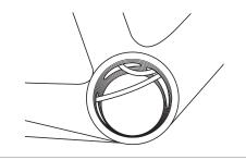
Set the electric wires so that only the electric wires for the front derailleur and the rear derailleur are visible inside the bottom bracket shell, and if any extra parts such as wire holders are protruding, push them back inside the frame.
