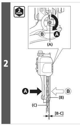
Use a 2mm hexagon wrench to turn the top adjustment bolt.
