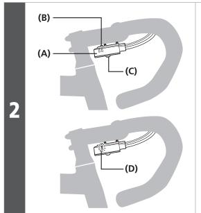
Press the button on junction A until the red LED illuminates in order to switch to adjustment mode.
