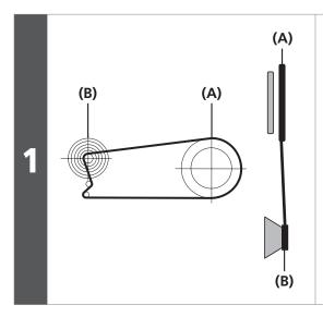
Set the chain on the largest chainring and the smallest sprocket.
