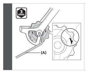
Replace pulleys using a 3mm hexagon wrench.
