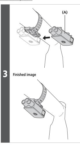
Slide SM-EW90 into the rail section of the hook to install it.
