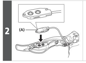
Place the switch unit onto the mounting surface of the setting plate.
