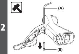
Place the lever with the shifting switch left side up as shown in the illustration.
