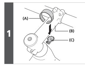
Attach to the stem using the band and hook included with SM-EW90.
