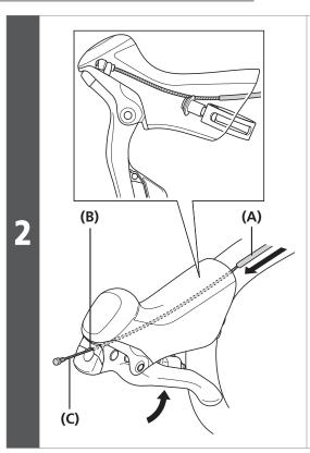
Depress the lever as if to brake and pass the inner cable through.
