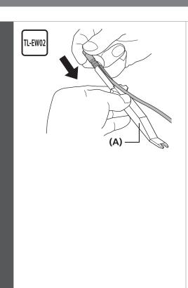
Set so that the projection on the connector is aligned with the groove on the narrow end.
