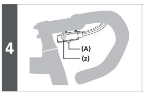
Press the button at junction A until the red LED turns off in order to switch from rear derailleur adjustment mode to gear shifting mode.
