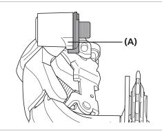
Hook the stopper plate on the stopper claw on the bracket body.
