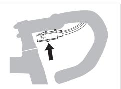
Press the button at junction A until the red LED turns off in order to switch from rear derailleur adjustment mode to gear shifting mode.
