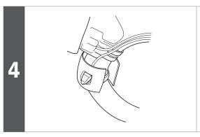
Align the hole in the handlebar tape which was cut with the switch.
