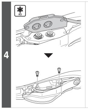
Make a gap between the switch unit and the setting plate and check that the end of the rubber on the switch unit is on the button.
