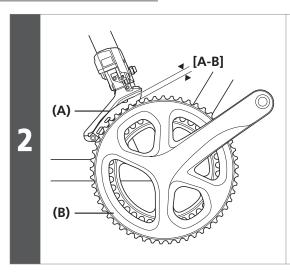
Adjust so that there is a clearance of 1 - 3mm between the chain guide outer plate and the largest chainring.
