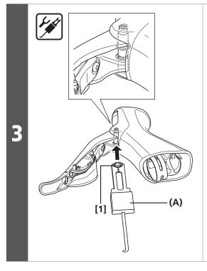
Use part [1] of the Shimano original tool to install the E-ring.
