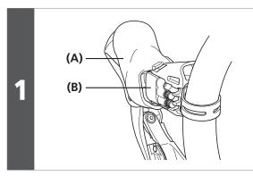
Open up the bracket cover and lift up the connector cover.
