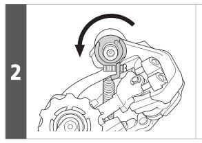
Use pliers to remove the stopper plate by moving it in the direction of the arrow.
