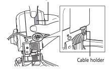
\* Using the wider end of the Shimano original tool TL-EW02, attach the electric wire on the cable holder.
