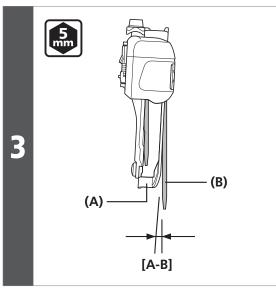
Use a 5mm hexagon wrench to secure the chain guide outer plate so that the flat part of the plate is directly above the largest chainring and so that the rear edge of the chain guide is within 0.5
