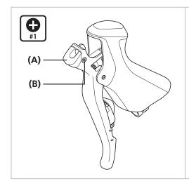
Grip the brake lever, remove the name plate mounting screws, and replace the name plate.
