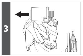
Remove the B axle seal ring and the B tension spring, then remove the B axle in the direction of the arrow.
