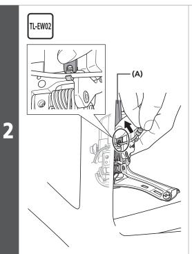
Remove the electric wire from the cable holder.
