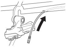
Electric wire for battery mount [In the case of an external battery (SM-BTR1)]
