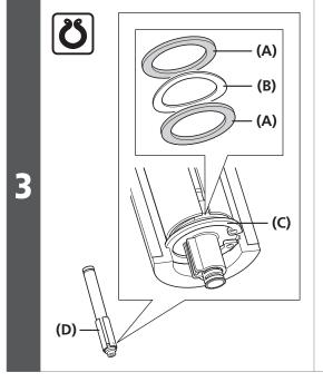
Mount a wave washer between two washers to the groove of the battery adapter, and fix them in place with a snap ring.
