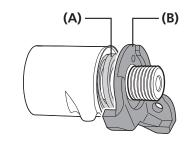
Temporarily assemble the B tension spring, B body seal ring, stopper plate and B axle to the B body.
