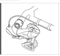
Temporarily secure the electric wire along the frame with tape, and connect it to junction B.
