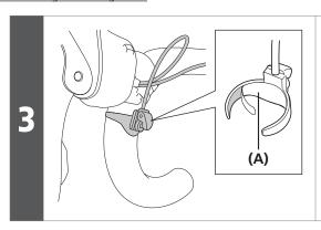
Make guide marks on the handlebars at the switch installation positions, and secure the switches with double-sided tape. (A) Double-sided tape
