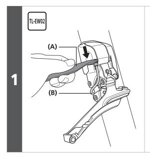
With the base portion of the hook firmly held down using the wider end of the Shimano original tool TL-EW02, remove the electric wire.
