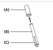
Insert internal battery into the collar from the bottom of seat post.
