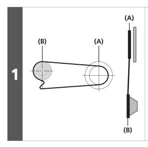
Set the chain on the smallest chainring and the largest sprocket.
