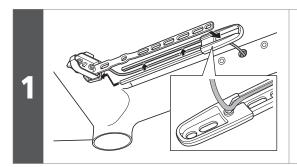
Set the electric wire for the battery mount into the groove in the electric wire cover for the battery mount.
