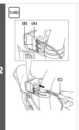
Use the TL-EW02 to connect the connector of the electric wire to the terminal on the lever side.
