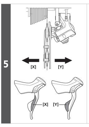
If shifting switch [X] is pressed once while the initial setting condition is active, the guide pulley will move one step toward the inside.
