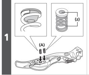
Check that the buttons are attached to the springs, then insert the switch springs into the holes in the switch unit setting plate.
