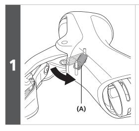
Assemble the bracket body and the lever body, and then attach the return spring.
