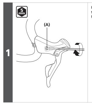
Peel back the bracket cover and tighten the clamp nut using a hexagon wrench.
