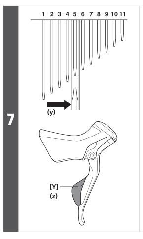
Next, operate shifting switch [Y] 4 times to move the guide pulley toward the outside by 4 steps to the target position.
