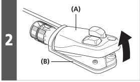
Remove the bracket cover from the end of the bracket.
