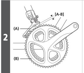
Adjust so that there is a clearance of 1 - 3mm between the chain guide outer plate and the largest chainring.
