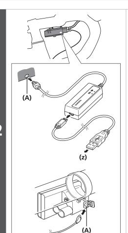
Connect the charging cable to the junction A or the charge port of the information display.
