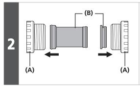
Install the inner cover to the bottom bracket adapter.
