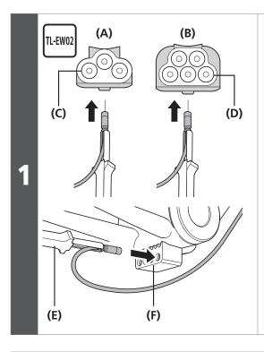
Connect the electric wires to junction A and junction B.
