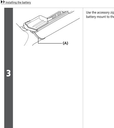
Use the accessory zip tie to secure the battery mount to the frame.
