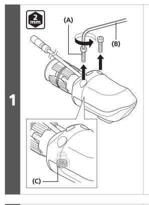
Remove two cover fixing bolts (M2.6) with a 2mm hexagon wrench.
