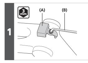
Remove the wire guide from the frame, if attached.
