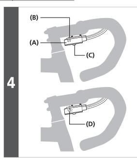
Press the button at the junction A until the red LED illuminates in order to switch to rear derailleur adjustment mode.
