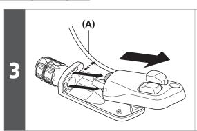
Disengage the two hooking tabs, and then remove the switch cable from the bracket groove.
