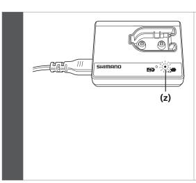
Remove the battery from the battery charger, disconnect the power plug of the battery charger from the electrical outlet, and then repeat the charging operation.
