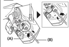
Shift to the smallest sprocket, and then tighten the top-side stopper bolt until it touches the left link at the position where the rear derailleur stops.
