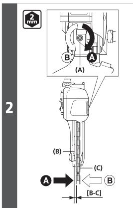
Use a 2mm hexagon wrench to turn the low adjustment bolt.
