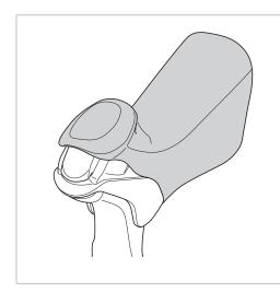
Always replace the bracket cover with the lever removed from the bicycle as shown in the illustration.
