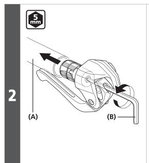
Install the brake lever to the handlebar by tightening counterclockwise with a hexagon wrench.
