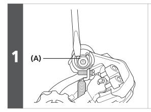
Remove the B axle stop ring using a slotted screwdriver.
