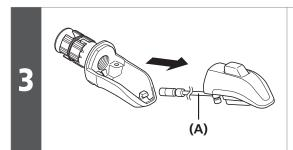
Disengage the two hooking tabs, and then remove the switch cable from the bracket groove. (A) Switch cable
