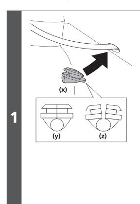
Install grommets in appropriate positions for the electric wires.
