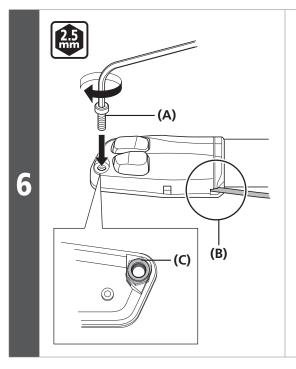
Check that the switch cable is protruding from the bracket groove, and then tighten the cover fixing bolt.
