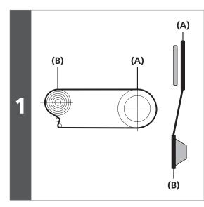
Set the rear derailleur to the largest sprocket.
