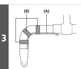
Temporarily secure the outer casing to the handlebar (by using tape or a similar material).
