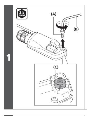
Use a 2.5mm hexagon wrench to remove the cover fixing bolt (M4).
