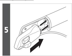
Insert the hooking tabs, match it up with the bracket cover to install the bracket.
