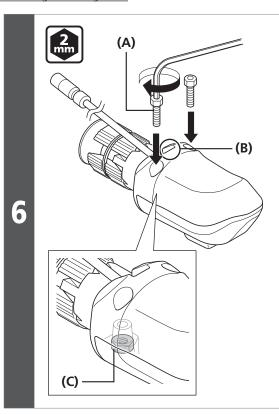
Check that the switch cable is protruding from the bracket groove, and then tighten the cover fixing bolt.
