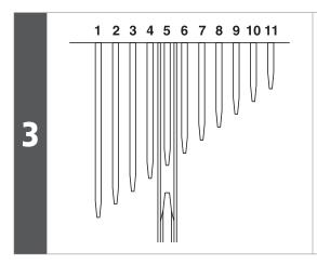
Shift the rear derailleur to the 5th sprocket position.
