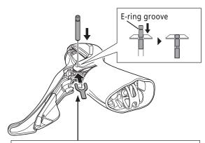
Do not press-fit the lever axle from this direction. Otherwise, it may damage the bracket body.
