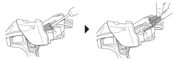
**3.** Before installing a new cable cover, make a slight crease on it and insert it into the hole in the bracket.
