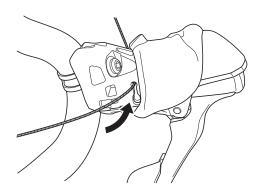
**3.** Insert the cable in such a manner that the inner end is attached to the unit.
