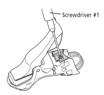
**2.** Remove the cable cover from the bracket using a screwdriver and pull the cable out with your hand.
