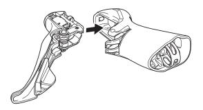
**2.** Insert the end of the return spring into the notch.
