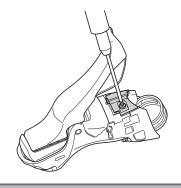
Tightening torque: 0.20 - 0.25 N⋅m {1.7 - 2.2 in. lbs.}
