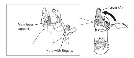
**3.** Rotate the main lever support in the direction of the arrow with a slotted screwdriver or an equivalent tool, and then remove the stopper.
