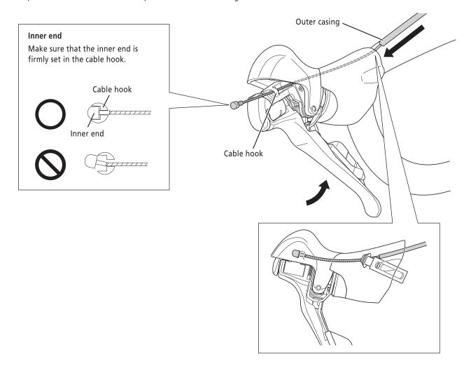
Temporarily secure the outer casing to the handlebar (by using tape or a similar material).
