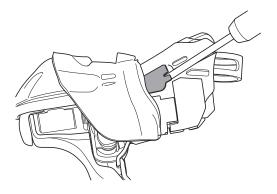
**3.** Use a pointed tool to pry out the SL cable guide.
