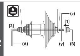
Tighten the fixing nut onto the hub axle [1] and then turn the hub axle [2] to secure the freehub to the frame.
