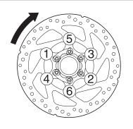
Wear gloves and turn the disc brake rotor clockwise with some force.
