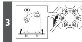
Use a slotted screwdriver or similar tool to bend the edges of the tightening plate over the heads of the bolts.
