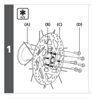
Install the disc brake rotor and the disc brake rotor tightening plate to the hub, and then install and tighten the bolts.
