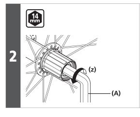
After removing the hub axle, remove the freewheel body fixing bolt (inside the freewheel body).
