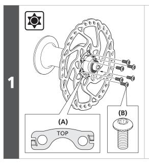
Install the disc brake rotor and rotor lock washers to the hub and tighten the bolts.
