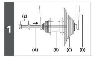
Install the sprockets to the freehub, place the freehub onto the frame and pass the hub axle through it.
