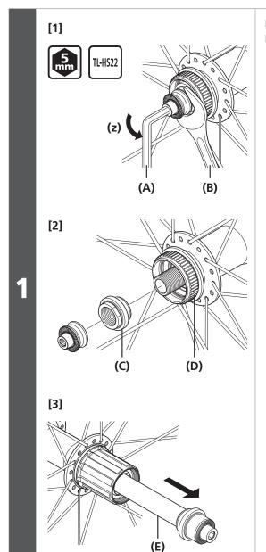
Pull out the hub axle by following procedures [1] to [3].
