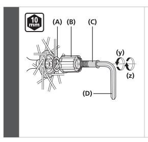
After removing the hub axle, remove the freewheel body fixing bolt (inside the freewheel body), and then replace the free-wheel body.
