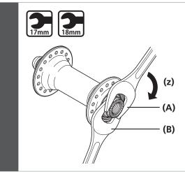
Install the hub axle, and then use hub spanners as in the illustration to tighten the lock nut so as to double-lock the mechanism.
