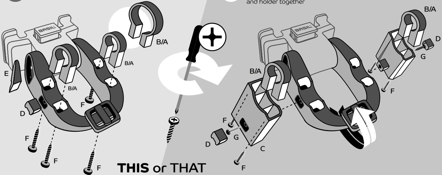
**3.** Close the velcro around the handlebar stem to avoid any movement and turn the head of the holder in the right angle
