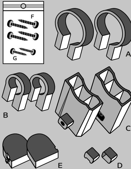
**1.** Check whether you need mounting bracket "A" or "B", depending on the diameter of the handlebar. Place the brackets on the handlebar
