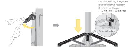
Close hook and slide to adjust to proper height. Open hook to lock in position.
