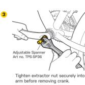
Use 8mm Allen wrench to tighten internal driver of extractor to remove crank arm.
