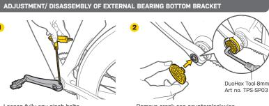
Remove crank cap counterclockwise.
