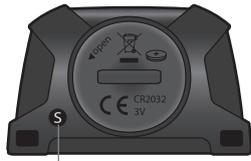
S Speed Sensor Sensing Point
