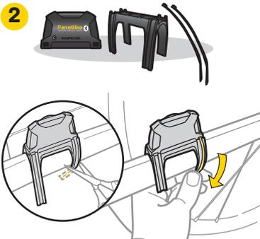
Pre-fit Sensor and Rubber Bracket on left rear chainstay (non-drive side) and trim excess rubber from bracket. Insure the Topeak logo is facing up. Install zip ties loosely to allow sensor placement.
