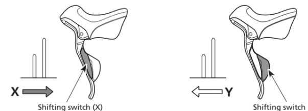
If the chain falls off on the inside, keep pressing shifting switch (X) for 1 second or more to move the front derailleur to the outermost position, and then keep it pressed for 10 seconds in order to reset the chain.
