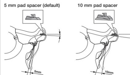
**Installation and removal of the pad spacer**
