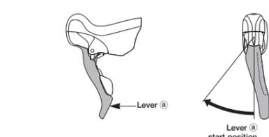
If operation of lever A dose not complete the chainring shift stroke, operate lever A again for the distance (X') to complete that part of the lever stroke (X) which was short.
