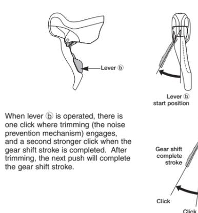
When lever B is operated, there is one click where trimming (the noise prevention mechanism) engages, and a second stronger click when the gear shift stroke is completed. After trimming, the next push will complete the gear shift stroke.
