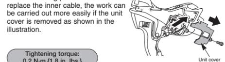
Be careful not to cover the cable holes or the unit cover when wrapping on the handlebar tape. If the handlebar tape covers these places, it will not be possible to replace the inner cable.
