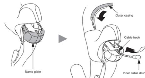
**Installing the shifting cable**
