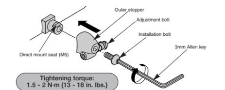
Install with the adjustment bolt tightened. The adjustment range for the adjustment bolt is six full turns.
