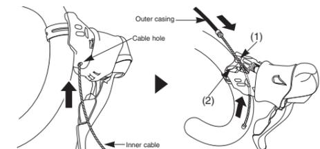
When removing parts in order to replace the inner cable, the work can be carried out more easily if the unit cover is removed as shown in the illustration.
