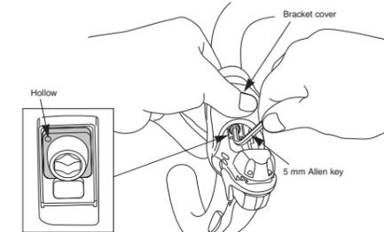
The correct way for clamp washer (B) to face is so that the small hollow on the surface is in the top-left corner.
