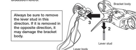
Always be sure to remove the lever stud in this direction. If it is removed in the opposite direction, it may damage the bracket body.
