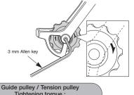
Tightening torque 2.5 - 5.0 N·m {22 - 44 in. lbs.}
