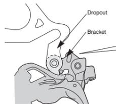
**Note:** Periodically check that there is no gap between the dropout and the bracket as shown in the illustration. If there is a gap between these two parts, problems with gear shifting performance may occur.
