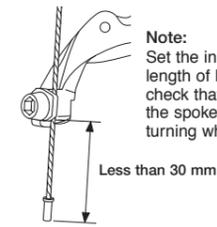
**Note:** Set the inner cable so that it protrudes by a length of less than about 30 mm, and then check that the inner cable does not interfere with the spokes of the wheel. Stop the wheel from turning while carrying out this step.
