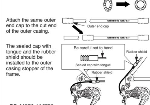
Attach the same outer end cap to the cut end of the outer casing.
