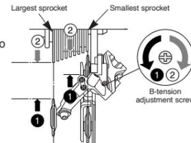
**<Checking the distance between the largest sprocket and the guide pulley>**
