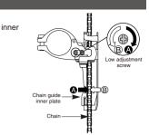
2. Connection and securing of cable While pulling the inner cable, tighten the wire fixing bolt with a 5 mm allen key to secure the cable.
